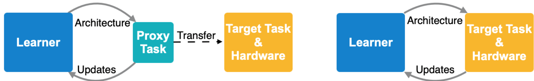
Figure: ProxylessNAS directly optimizes neural architecture on target task and hardware.
